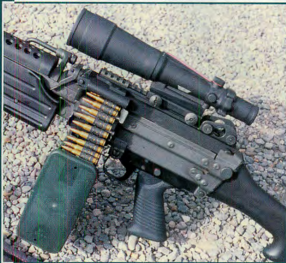
Trijicon's brand-new TA55 ACOG scope proved very effective on the M249. Designated the T9 in U.S. Army tests, the first MINIMI won the Squad Automatic Weapon Competition in 1974, and went on to be adopted as the M249 SAW.
